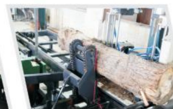
自动翻料，提高原木出材率 Automatic log turner, increase outturn rate.
